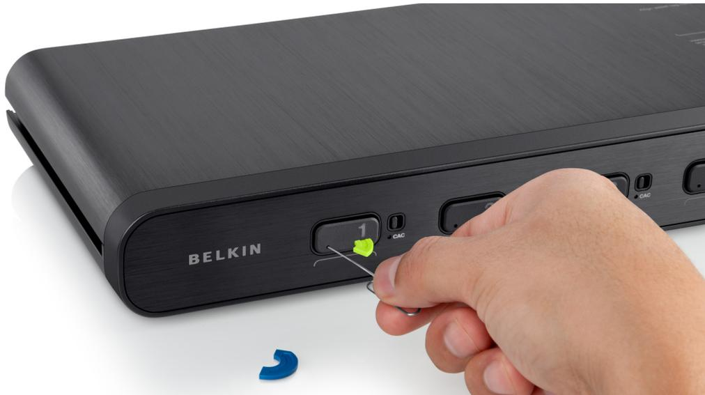
Belkin minimizes user error by incorporating customizable color-coded ports with labels that to associate the port with the network. The switches' port button is illuminated to indicate the specific computer the console is controlling.
